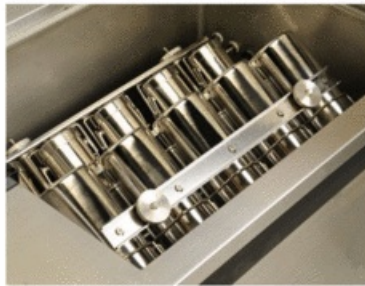
Small beakers containing 200g of washing solution, steel balls, test samples
