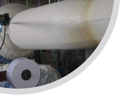
**Spray** production is particularly suited for medium to large diameter pipes and regular to heavy weight pipes. Rotating spray insulation of pipes provides economic advantages thanks to the possibilities to use thinner outer casing and improved productivity thanks to shorter set-up times when changing the pipe diameter.
