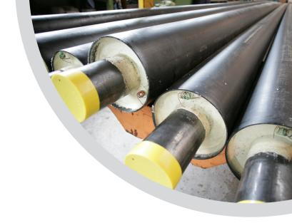
**Straight pipes** are pipe-in-pipe systems with an inner pipe that is usually made of steel and they account for the majority of pre-insulated pipe applications. Standard lengths for pipes are 6, 12 and 16 meters and specialty variants of straight pipes include **curved pipes** and **fittings** that allow directional changes of the pipe run.
