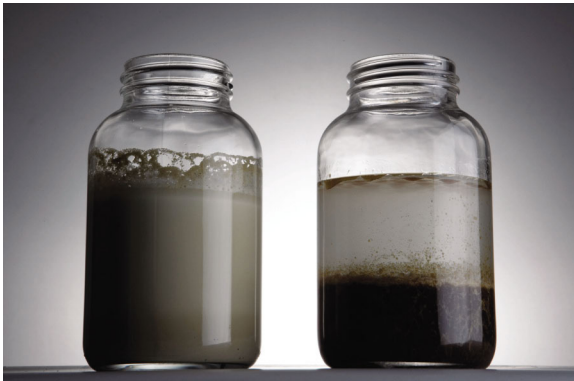
Figure 14. Comparative photograph: dispersions of isocyanates in water after standing for 40 minutes. The image on the right shows the instability of standard isocyanates while the image on the left shows the emulsion stability of emulsifiable isocyanates.
