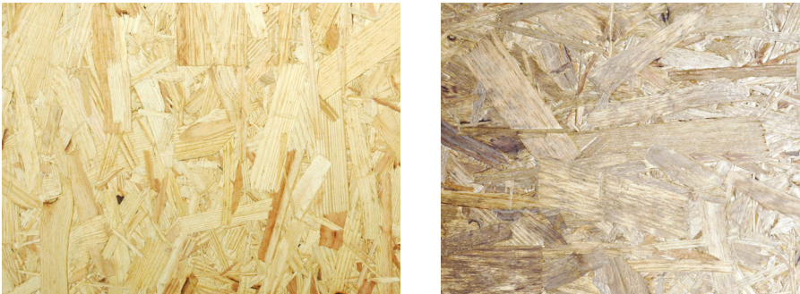
Figure 11. Surface color of soap released OSB panel (right) and new development releasable isocyanate technology (left).
