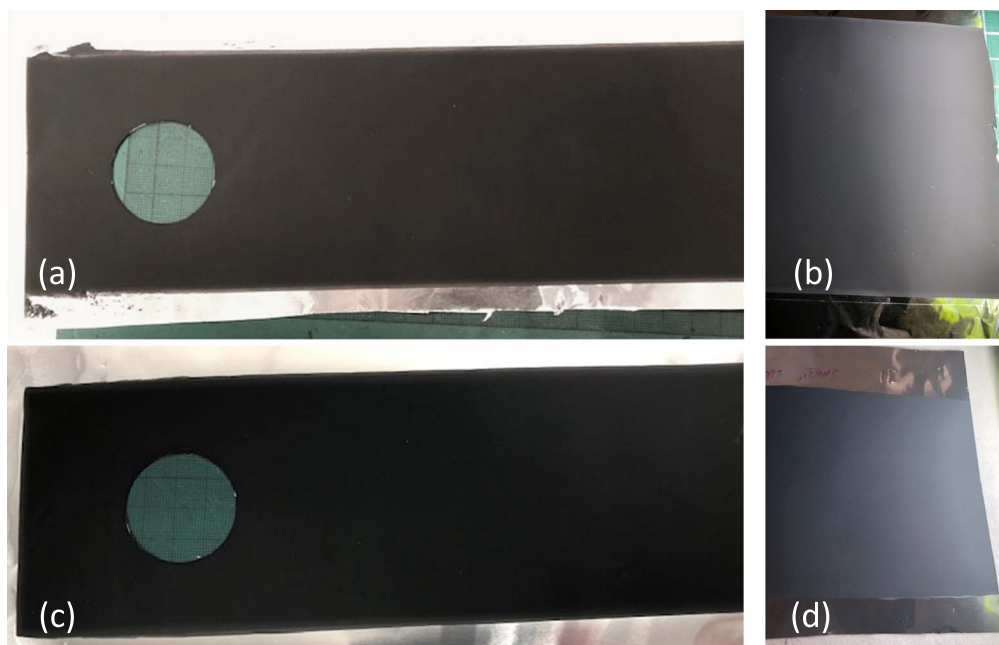
Figure 2. Photographs to show coatings made from the JEFFSOL® MEOX and NMP based slurries. (a) A 200 GSM uncalendered coating formed from a JEFFSOL® MEOX slurry. (b) A JEFFSOL® MEOX-formed coating photographed under illumination, to show that no visible aggregates are present. (c) A 200 GSM uncalendered coating formed from an NMP slurry. (d) An NMP-formed coating photographed under illumination to show that no visible aggregates are present.
